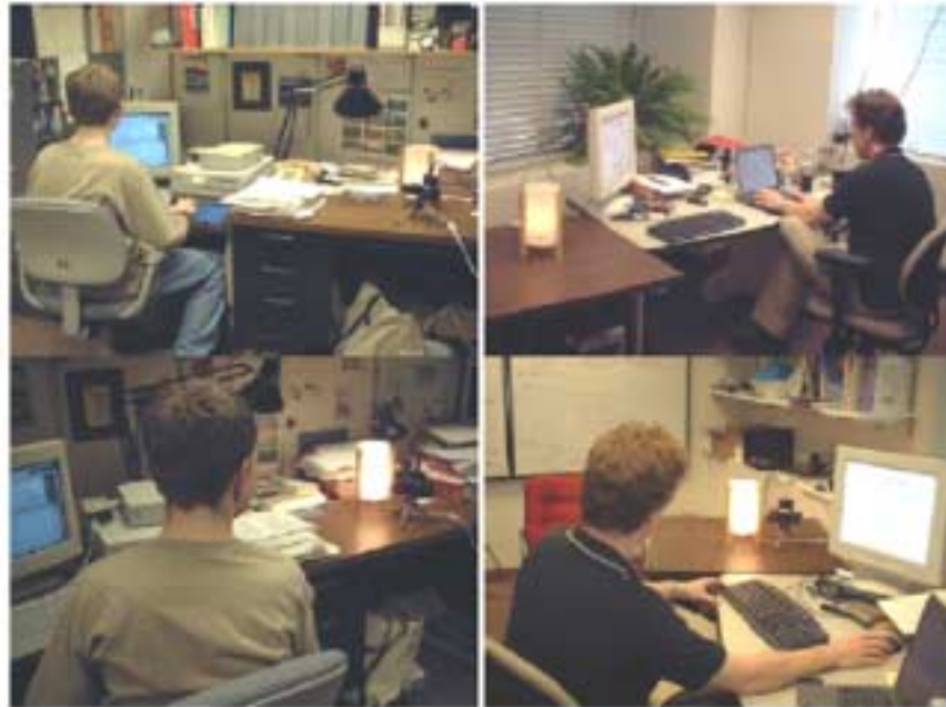
Figure 1-2: The usage of the Perceptive Presence Lamp. In the top row, both users are working, and their lamps are dim. In the bottom row, the user on the right has looked at his lamp (much as a person would look at an office mate to get their attention) thus brightening the lamp at the other location. This brightening got the user on the left's attention and he returned the glance to the user on the right.
