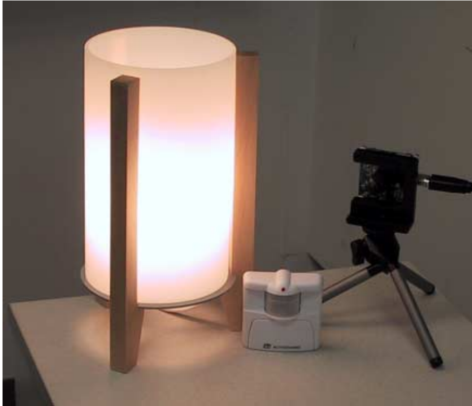
Figure 1-3: The original Perceptive Presence Lamp prototype. This lamp used an X10 motion sensor to determine if a person was present and a camera running a face detector in a subset of the field of view to determine if a person was trying to send a glance using the lamp.
