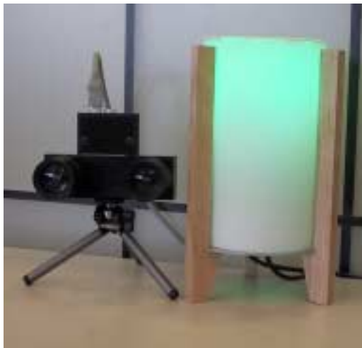
Figure 5-1: The color changing Perceptive Presence Lamp uses a stereo camera and the Spatial Selection Widget to determine where people are located and conveys this information to a remote location through of color on a lamp.
